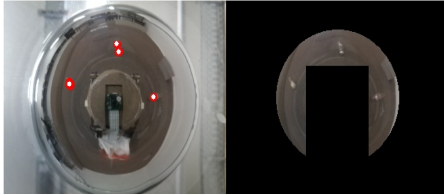
Figure 29: Bottle detection using OpenCV. Right side shows the mask along with bottles in the arena. Left side shows the bottle detected by the algorithm. Contours indicated in red color, Centroid of the contour indicated in white color
