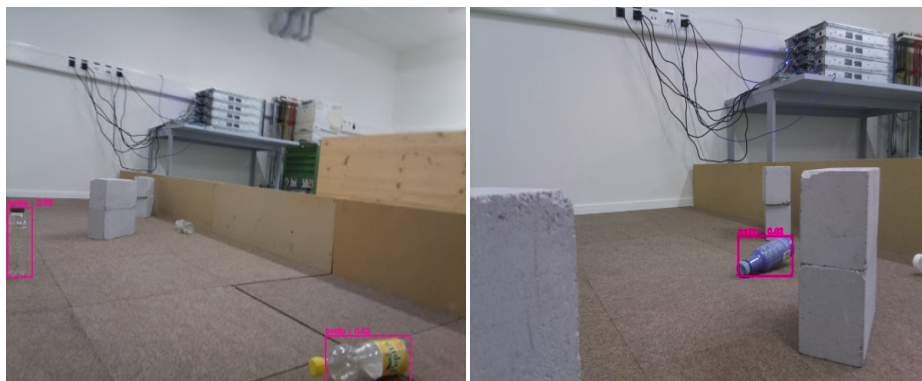
Figure 28: Bottle detection using deep learning in OpenCV
