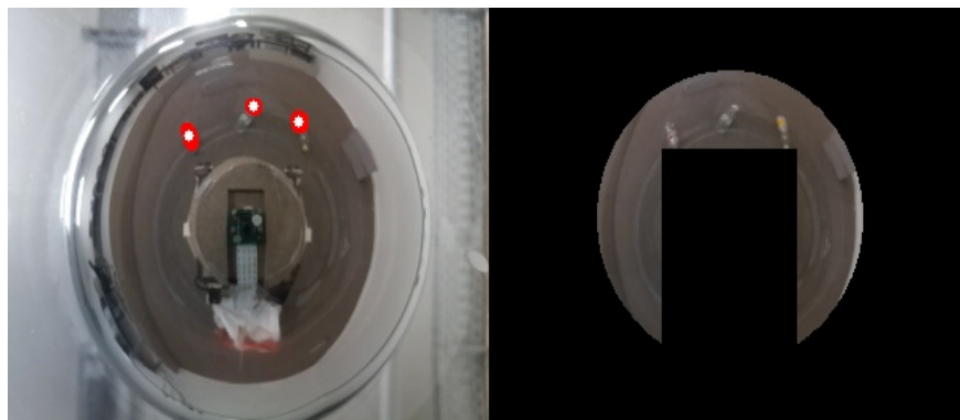
Figure 31: Bottle detection using OpenCV. All bottles in front.
