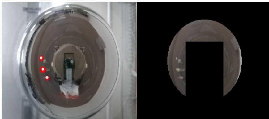
Figure 30: Bottle detection using OpenCV. All bottles to the left.
