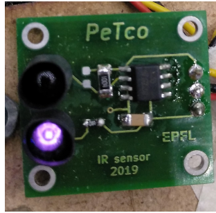
Figure 13: PCB of the custom IR sensor once received and soldered (We can see well the infrared light as the quality of the smartphone camera is poor)
