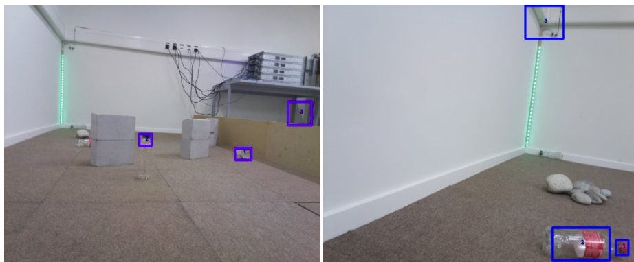
Figure 27: Bottle detection using image processing with OpenCV
